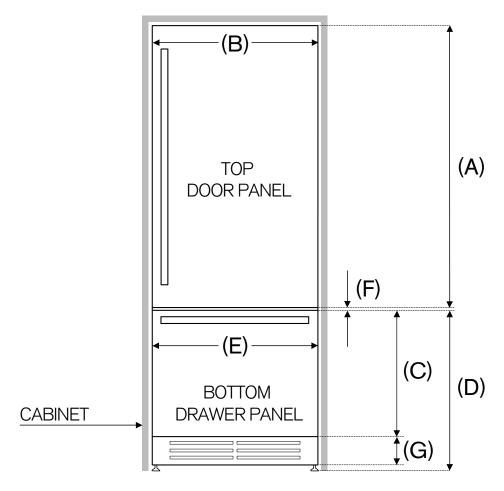
**NOTE**: These specifications assume a standard toe kick height of 100 mm. For different toe kick heights, adjust C accordingly.
